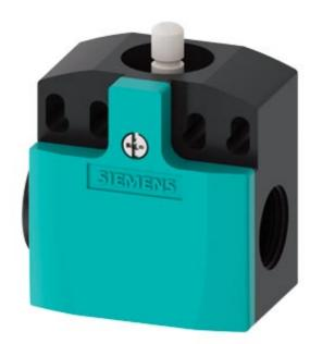
Position switch Plastic 50 mm Increased corrosion protection Device connection 2x (M20x 1.5) 1 NO/1 NC quick action contacts Rounded plunger functional at -40  $^{\circ}$ C Shock and vibration test according to EN 61373, Category 1B
