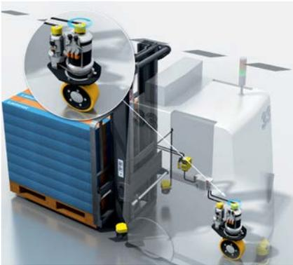
With automated guided systems (AGS), the SSM (safety speed monitor) or SLS (safety-limited speed) function monitors the speed on the wheels using the DFS60S Pro encoder and reduces it via the controller if necessary. Thanks to a
