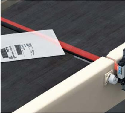
The leading edge detection serves to convey objects at a specified distance from the belts to the main sorter. The combination of high-resolution light grids and high-resolution encoders allows leading edge detection and the detection of additional object profile information such as the length.
