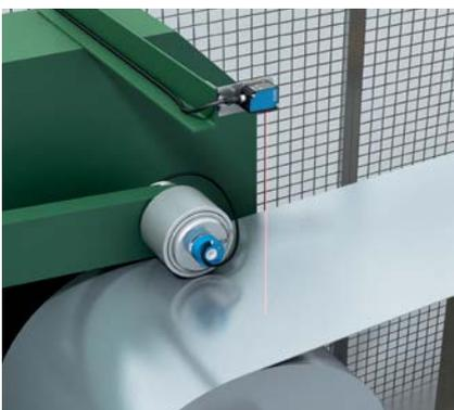
To ensure a constant feed of material, the uncoiling speed of the sheet coil must be regulated. The distance sensor continuously measures the radius of the sheet coil throughout the entire unwinding process. The DBS60 Core incremental encoder uses a friction roller to mea-
