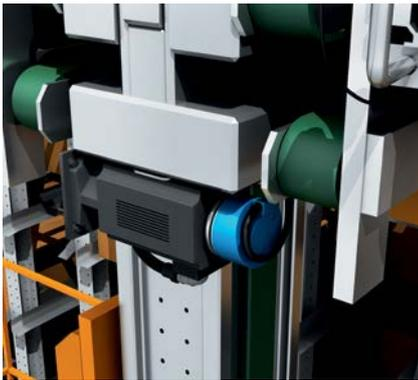
When it comes to the insertion depth, accurate measurements are crucial. A rugged absolute encoder on the belt drive with a high resolution and excel-
