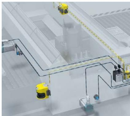
The movements of the CNC portal, which the worker cannot predict and which can be very rapid, represent hazardous points during the machining process. The modules of the Drive Monitor FX3-MOC safely monitor the electric drive system of the CNC plasma cutting machine in conjunction with the signals of the Flexi
