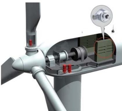
Generally, incremental encoders are used to monitor the rotor speed. These are normally fastened to the hub of the rotor. The DFS60 incremental encoder is used around the world under the harshest conditions. Its stable construction with enclosure rating up to IP67 makes
