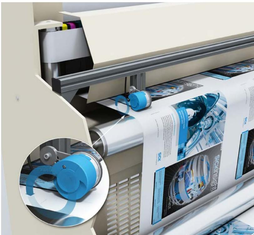
Incremental encoders detect the speed of the print media and provide key information on the correct position for the print and the quality of the printed image. Whether you require clearly legible bar codes or high resolution printed check cards, gift cards, or brochures – accurate speed monitoring ensures print quality.
