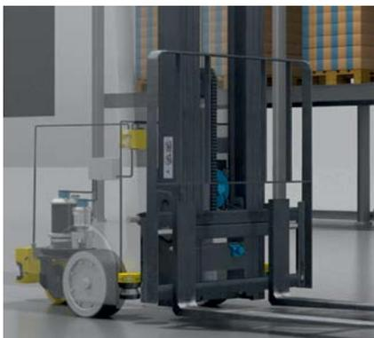
The measurement of the fork lifting height on the AGS for the precise removal of print products from the bay is
