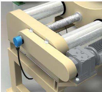
The positioning of saw-blades for setting to the thickness to be sawed is carried out with the ATM60 absolute encoder.
