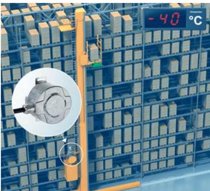
To avoid an unnecessary increase in enormous cold store energy requirements, it is important to ensure optimal storage and retrieval. Among other things, this depends on accurate and above all, reproducible positioning of the
