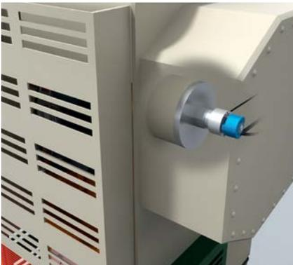
An ATM60 absolute encoder is mounted to the eccentric shaft on mechanical presses for the purpose of determining the position of the press stroke. It reli-
