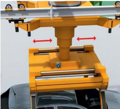
The electrical overhead conveyor brings the car bodies to designated workplaces. The speed is specified by the higher-level control; an incremental encoder determines the speed. In case of require-
