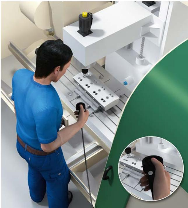
Stationary machines are often equipped with mechanical solutions, such as doors or flaps, to separate the user from hazardous points. When working on machines in maintenance or setup mode, the safe speed monitor reduces the risk of injury and increases productivity.
