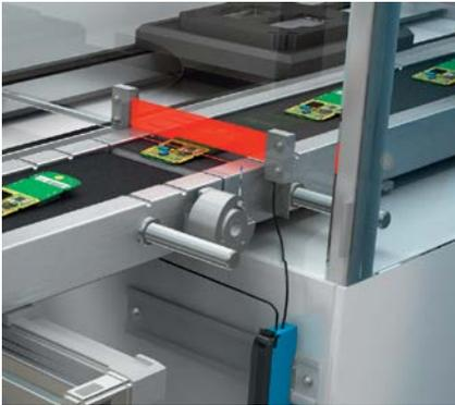
The DBS60 Core incremental encoder transfers the position of the belt for synchronization of both sensor signals. Alternatively, the belt speed can be taken
