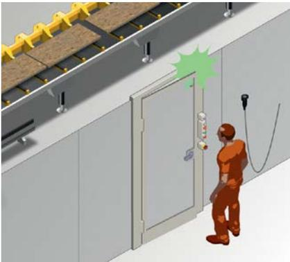
On the saw line, the operator is kept away from the hazardous point by a safety fence. In order to eliminate faults on the line, a safe standstill detection is necessary or for the maintenance and
