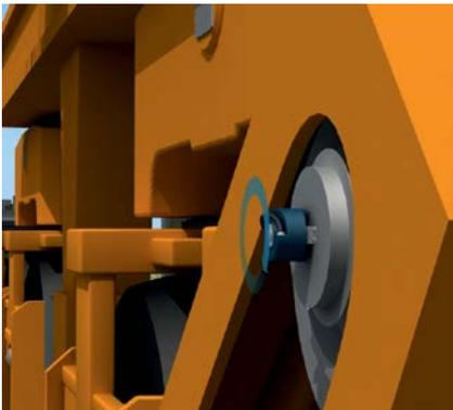
The speed of the drive motor of a crane is measured with the DBS60 incremental encoder. This way, the speed can be con-
