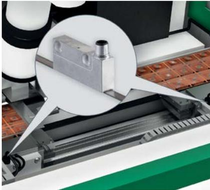
Temperatures are very high in the area around the bonding head, making fiber-optic cable systems the most effective for this application. With its 16  $\mu$ s response time, the WLL180T works together with the LL3-TH fibers to supply the control unit with a precise signal for edge detection. The grippers of the wire
