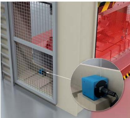
To determine the position of the press stroke, a BKS wire draw encoder is used. It reliably supplies signals for estab-
