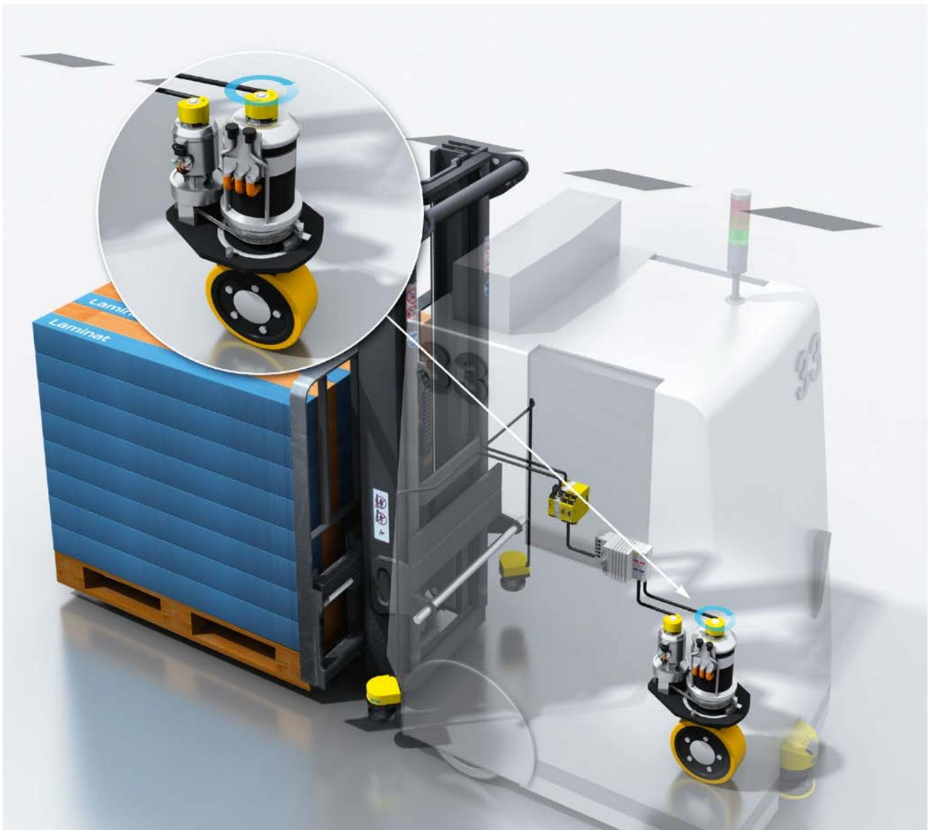
The safety encoder provides information on the speed and rotational direction of the driver and thus on the speed and direction of the automated guided system. As shown here, the encoder can be installed directly on the motor or, alternatively, on an axle. Hollow shaft encoders are normally used for automated guided systems.
