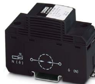
Single-channel, encapsulated, N-PE spark gap, 100 kA lightning test current, for Lightning Protection Level 1
